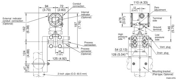
\*1: When Installation code 2, 3, or 8 is selected, high and low pressure side on above figure are reversed. (i.e. High pressure side is on the right side.)
