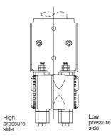
Horizontal Impulse Piping Type (INSTALLATION CODE '9') (For CODE '8', refer to the notes below)
