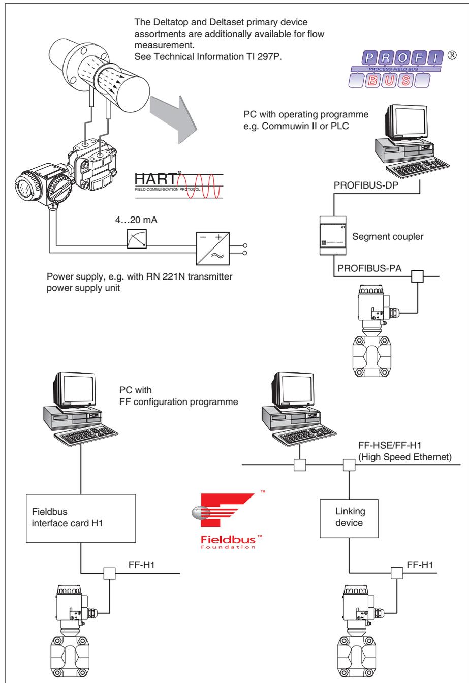
Complete measuring system Deltabar S
