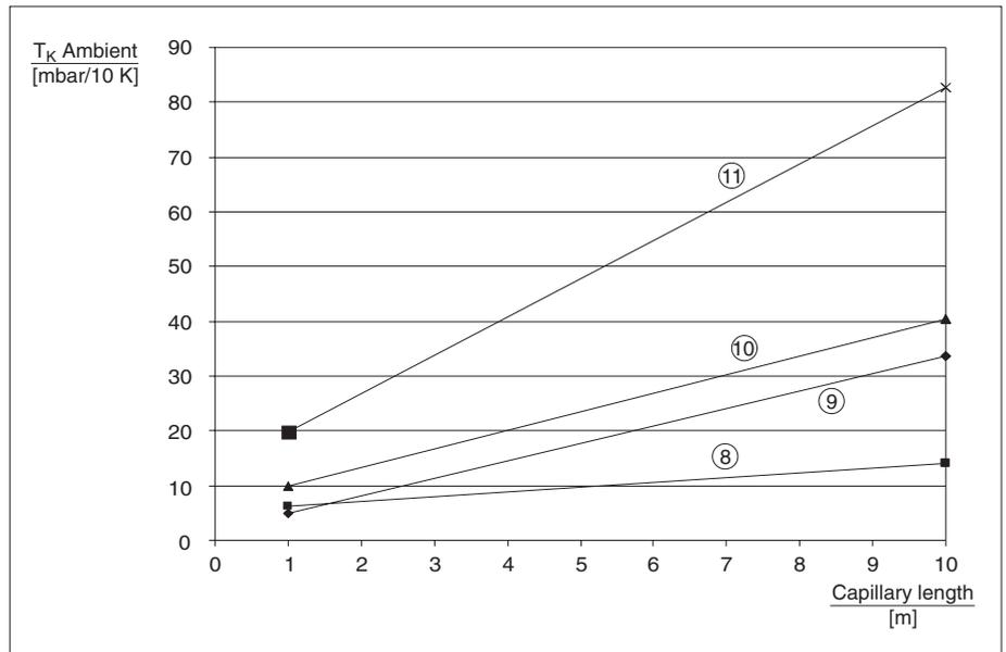
Diagram  $T_K$  Ambient dependent on the capillary length for FMD 633
