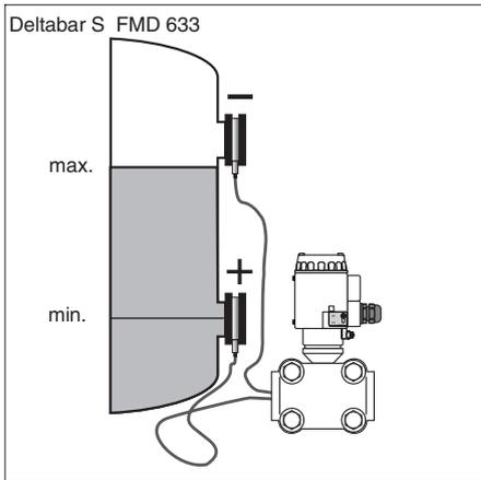
**Capillary diaphragm seal:**
