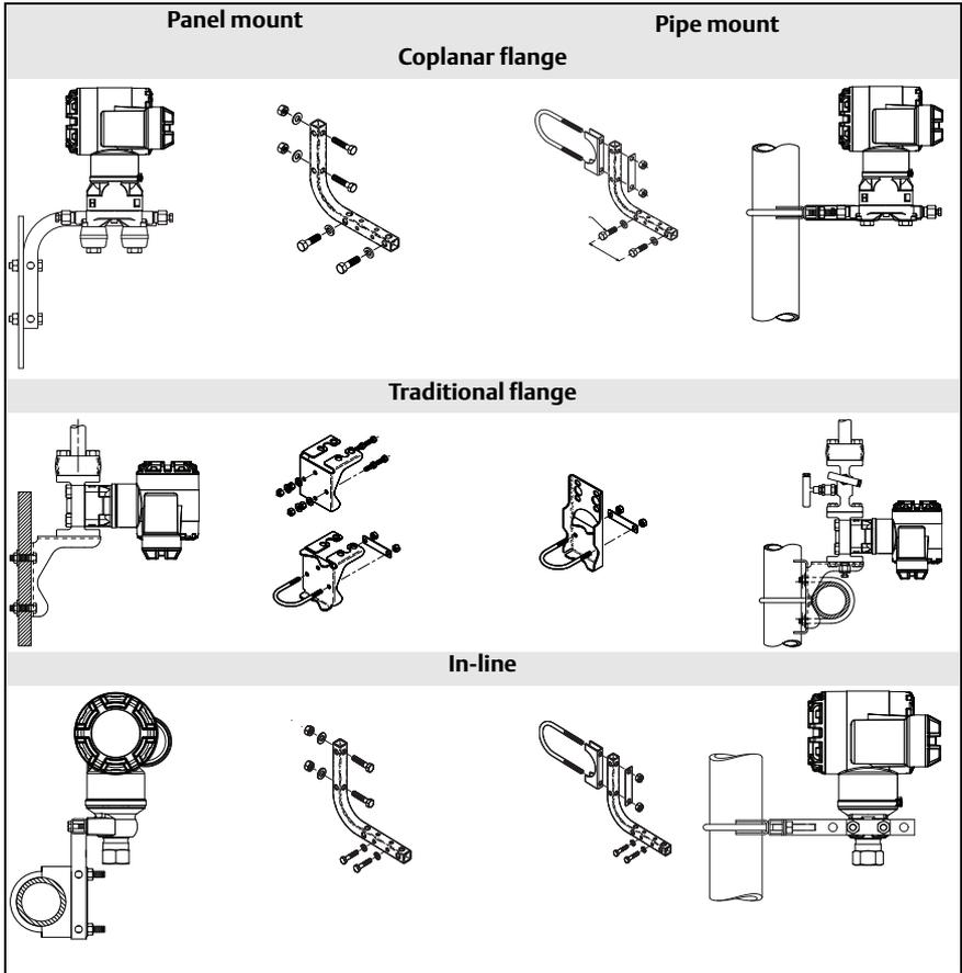
**Figure 5. Common Transmitter Assemblies**
