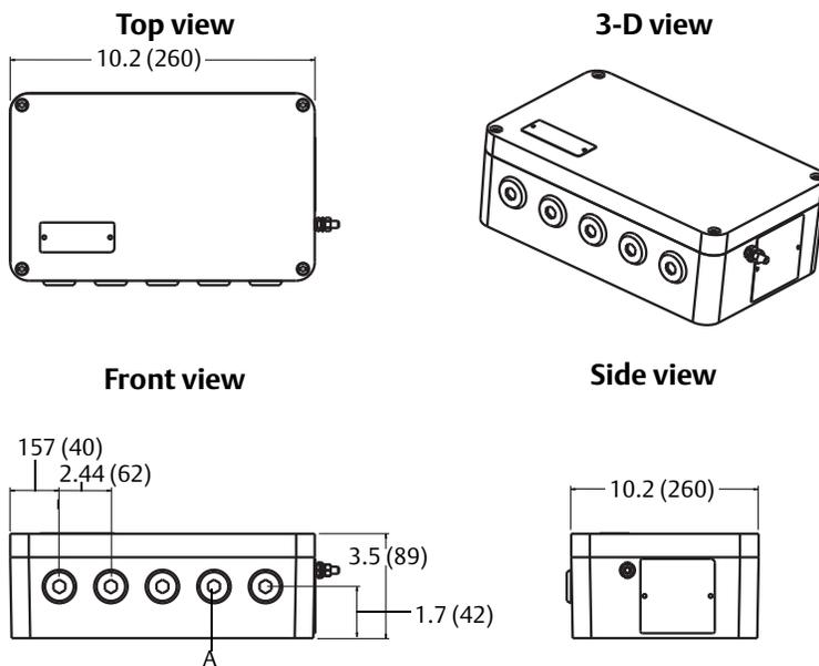
A. Five Plugged 0.86-in. diameter holes suitable for installing 1/2-in. NPT fittings
