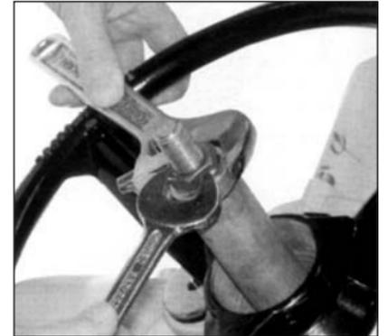
Fig. 5.6 Down Stop two Spanners
