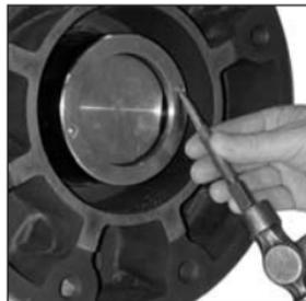
Fig. 4.6 Removal of Retainer
